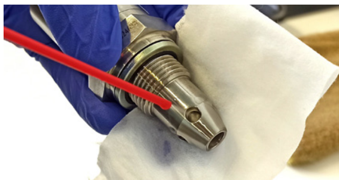
Fig. 4-1 Cleaning the Sensor
