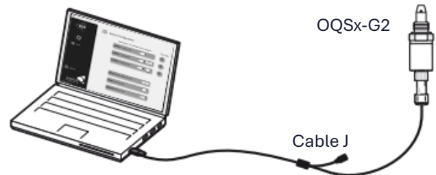
Fig. 4-2 Setting up a sensor for configuration
