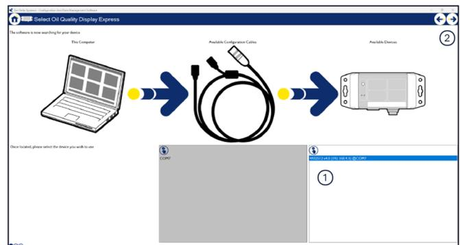
Fig. 3-1 QQDe selection screen in CADS
