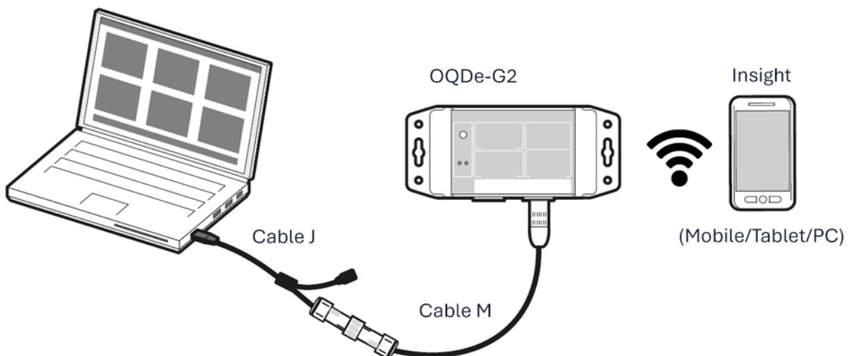
Fig. 4-1 Connecting to the OQDe-G2 via Wi-Fi Hotspot
