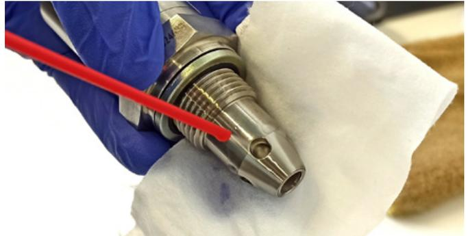
Fig. 9-1 Cleaning the Sensor
