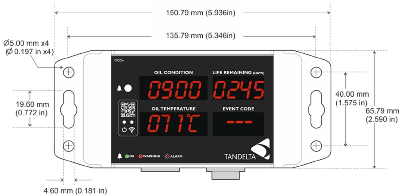
Fig. 6-1 OQDe-G2 Mounting Dimensions
