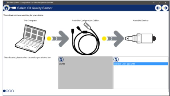
Fig. 2-2 CADS Sensor selection screen
