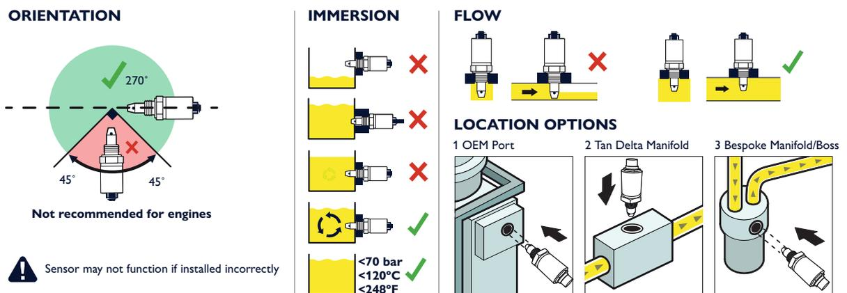
Fig. 5-2 Choosing a mounting location for the Sensor
