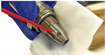
Fig. 5-1 Cleaning the Sensor
