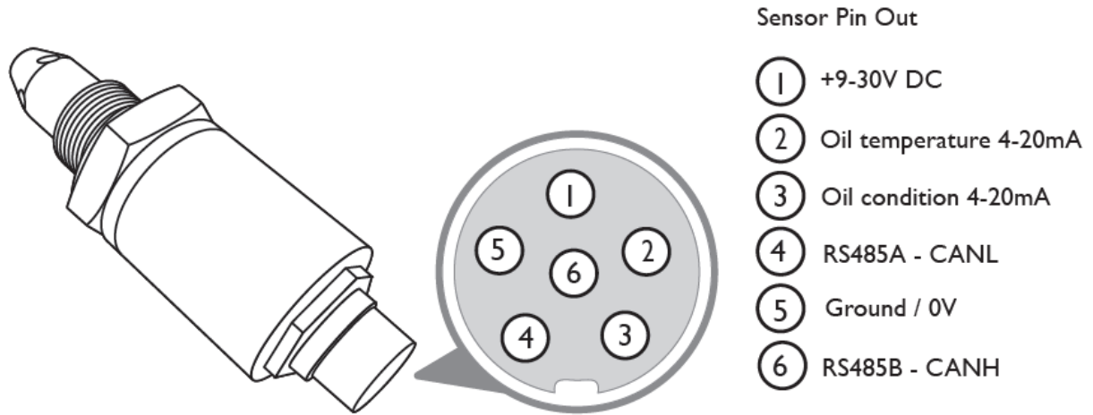
Figure 11 - Pin Outs for Power Supply & Data Output
