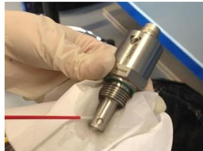
Figure 85 - Cleaning the Sensor (1)
