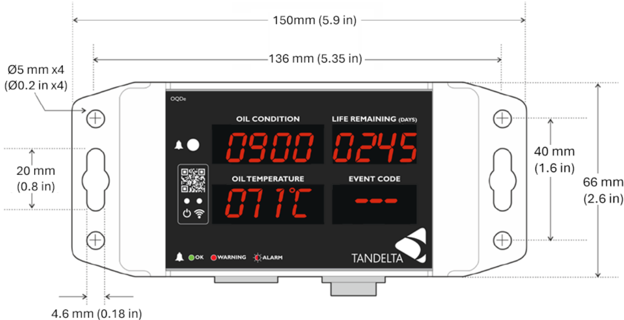
Fig. 6-1 QQDe-G2 Mounting Dimensions
