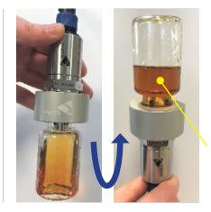
**Step 2:** Check red fibre washer/seal is in place in the bottle adaptor. Pour your oil sample into a clean sample bottle and screw onto the bottle adapter. Agitate for a few seconds and invert the whole assembly.
